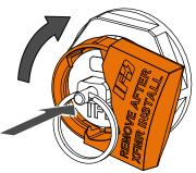
Ensure that the Shipping Lock is installed with **both tabs engaged**.
