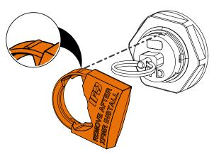
Push Shipping Lock and rotate clockwise to engage.
