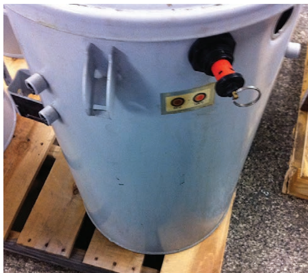
This transformer was returned to the shop after failing in the field. The IFD has popped and the exposed red is easily visible, even from the ground.
